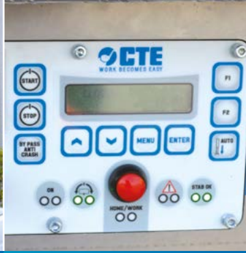
DIAGNOSTIC TOOL INTEGRATED IN THE CONTROL PANEL
